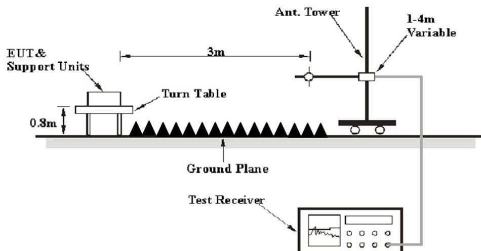
The radiated emission tests were performed in the 3 meters chamber test site, using the setup accordance with the CISPR16-1-4:2010+A1:2012, CISPR 16-2-3:2010+A1:2010+A2:2014. The limit was specified in EN 55032 Class B.
