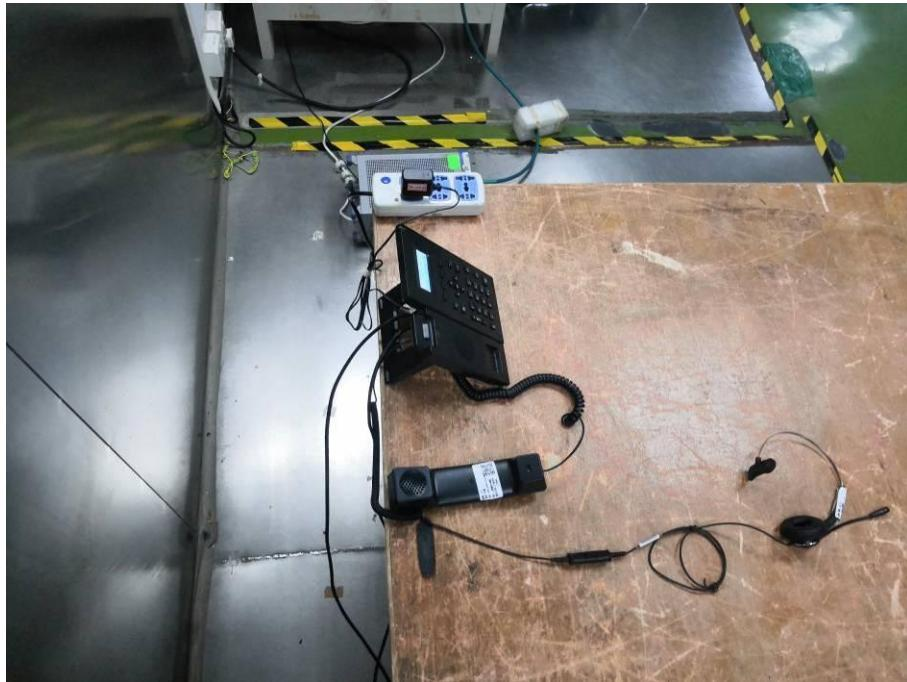
**Conducted Emissions - Front View (Powered by Adapter 2)**
