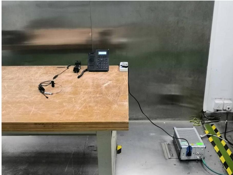
**Conducted Emissions - Side View (Powered by Adapter 2)**
