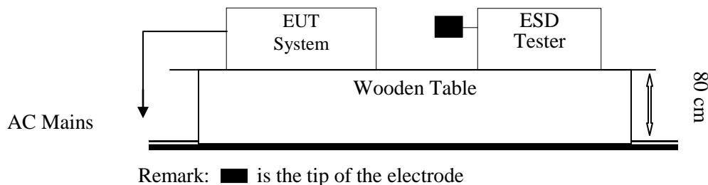
IEC 61000-4-2 specifies that a tabletop EUT shall be placed on a non-conducting table which is 80 centimeters above a ground reference plane and that floor mounted equipment shall be placed on a insulating support approximately 10 centimeters above a ground plane. During the tests, the EUT is positioned over a ground reference plane in conformance with this requirement.
