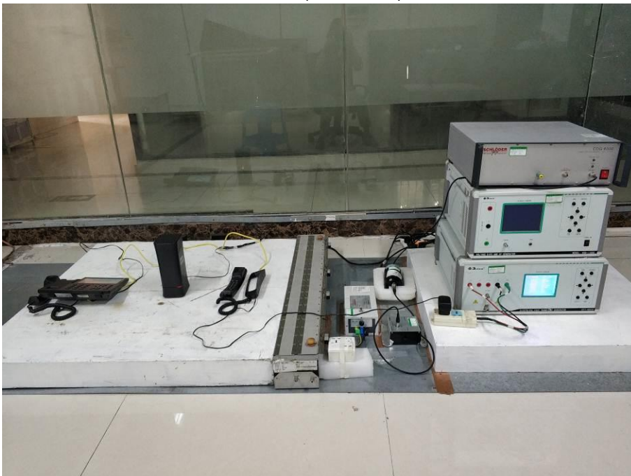
Electric Fast Transients(AC Mains) for Test mode 1
