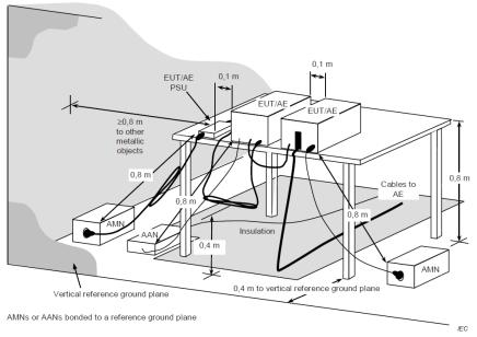
The 0.8 m distance specified between EUT/AE/PSU and AMN/AAN, is applicable only to the EUT being measured. If the device is AE then it shall be  $\ge$ 0.8 m.
