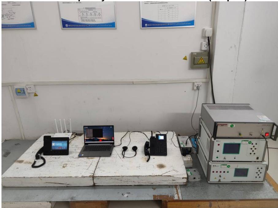
**Radio frequency continuous conducted (Signal port)**
