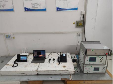
Radio frequency continuous conducted (Signal port)
