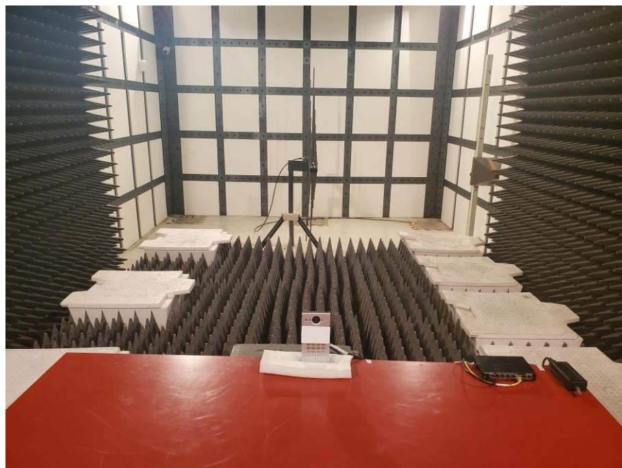
**RS Test Setup Photo (Above 1GHz)**
