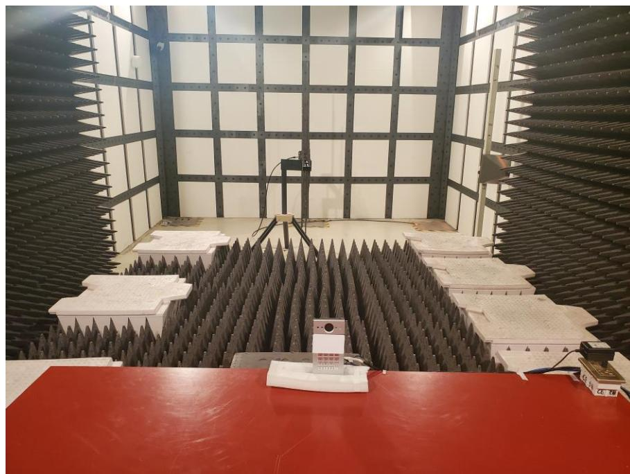
**RS Test Setup Photo (Above 1GHz)**
