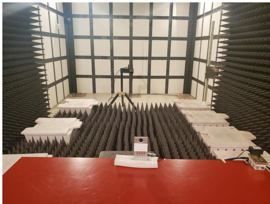
**RS Test Setup Photo (Above 1GHz)**
