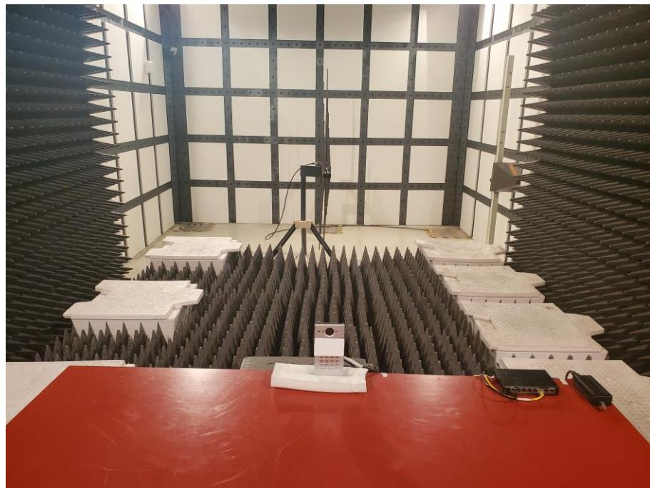
**RS Test Setup Photo (Above 1GHz)**
