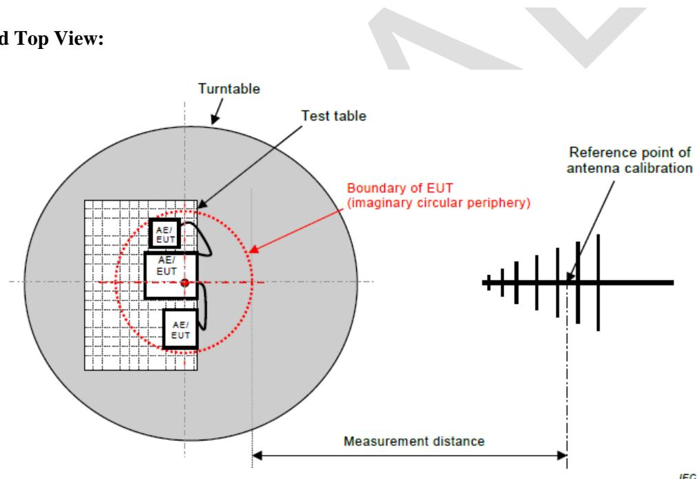
**Figure C.1 – Measurement distance**
