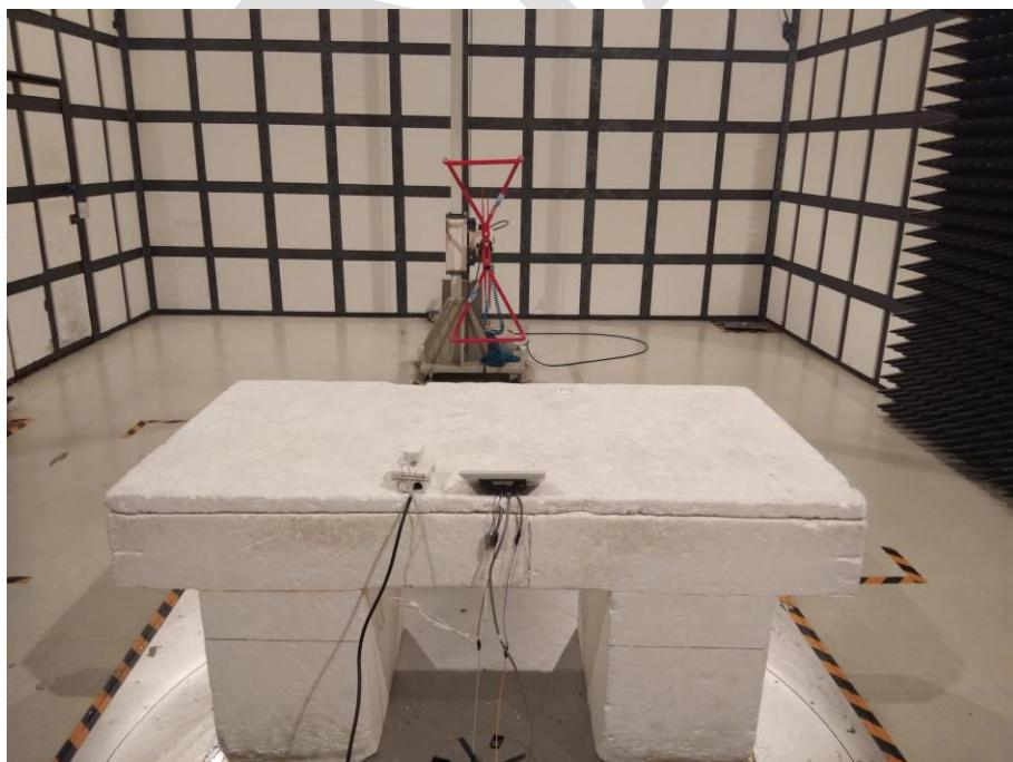
**Radiated Emissions - Rear View (Above 1GHz)**
