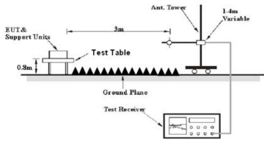
**Radiated Top View:**
