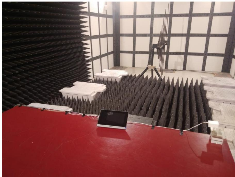
**RS Test Setup Photo (Above 1GHz)**
