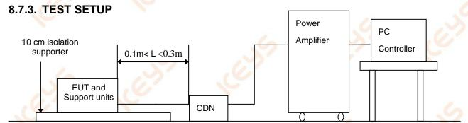
For the actual test configuration, please refer to the related item – Photographs of the Test Configuration Note: 1) The EUT is setup 0.1 m above Ground Reference Plane
