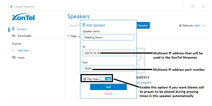
3. Assign the same Multicast IP address and Multicast port number in the IP phone or IP speaker that you set in XonTel Streamer application to start broadcasting the the audio in this IP phone or IP speaker from XonTel Streamer.
