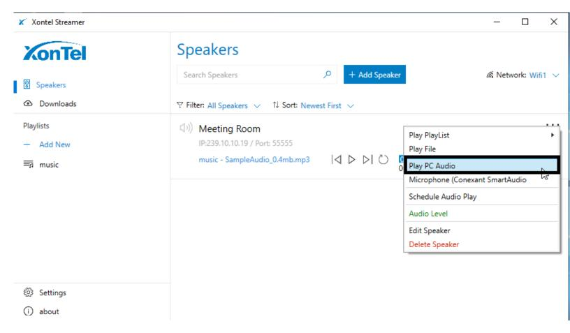
D. Broadcast the audio by using PC Microphone (You can talk from PC microphone and this sound will be broadcasted in the speaker).
