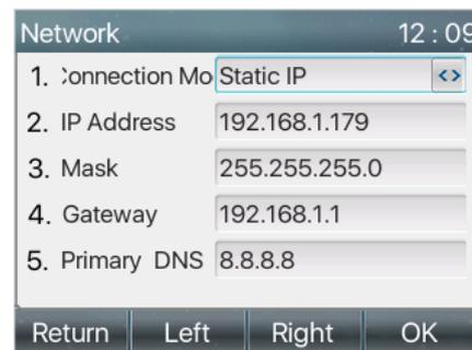
**Picture 112 - Static IP network mode**
