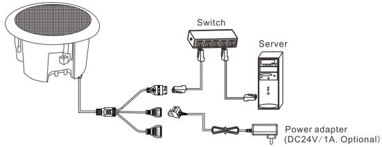
Note: POE switcher can not be connected, when using power adapter.
