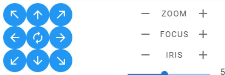
**PTZ control:** Eight direction keys can control the rotation of front-end equipment, and the middle is automatic rotation
